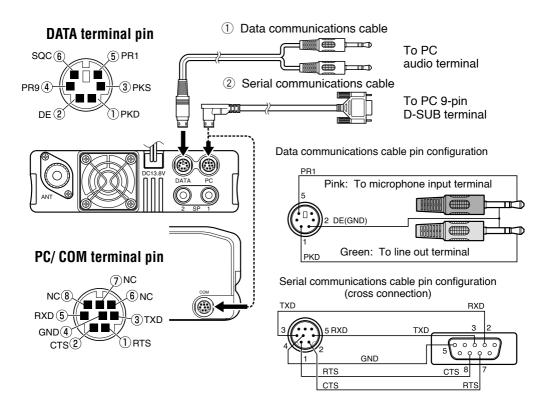
**Note:** When connecting the regular cable in your vehicle, the terminal may disconnect due to vibrations. Be sure to lock the cable in place.
