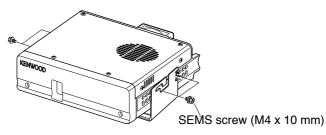
Set an appropriate angle for the TX/ RX unit, using the 3 screw slots on the rear edge of each bracket side.
