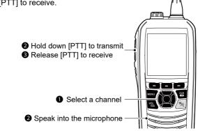
**TIP:** To maximize the readability of your transmitted signal, pause for a second after pushing [PTT] and hold the microphone 5 to 10 cm (2 to 4 inches) from your mouth, and then speak at your normal voice level.
