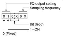
You can set the I/Q signal output setting by sending the command through the [I/Q OUT] port.
