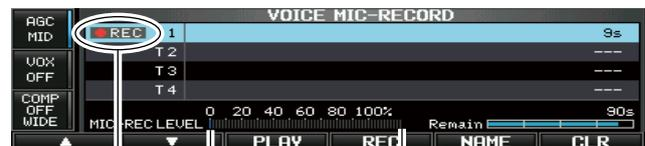
Appears Adjust **[MIC GAIN]** control so that this indicator reads within 100%.
