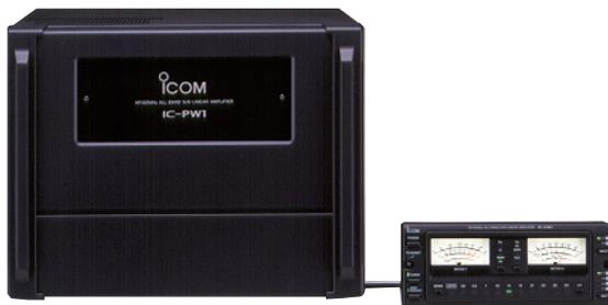
Full-duty 1 kW linear amplifier including an automatic antenna tuner. Has automatic tuning and band selection capability. Full break-in (QSK) operation is possible. The amplifier/power supply unit and the remote control unit are separated. An optional OPC-599 is required for connection.
