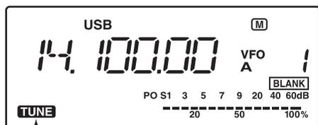
Appears when the antenna tuner is ON.
